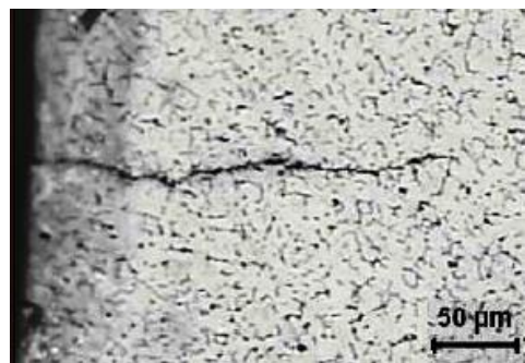
Figure 7 Crack deflection in weld metal 873 K
