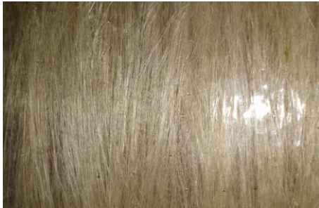
Fig 3.1 One Banana and a Glass Fiber Composite
