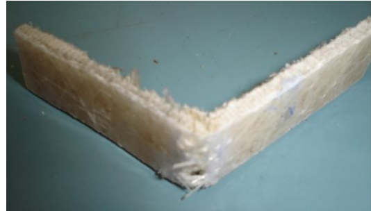
Fig. 4.5 Flexure Failure of the Specimen
