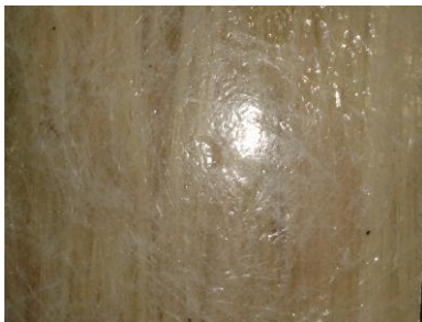
Fig. 3.2 Two Glass Fiber and a Banana Fiber
