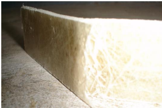
Fig.4.9 Impact Failure of the Specimen
