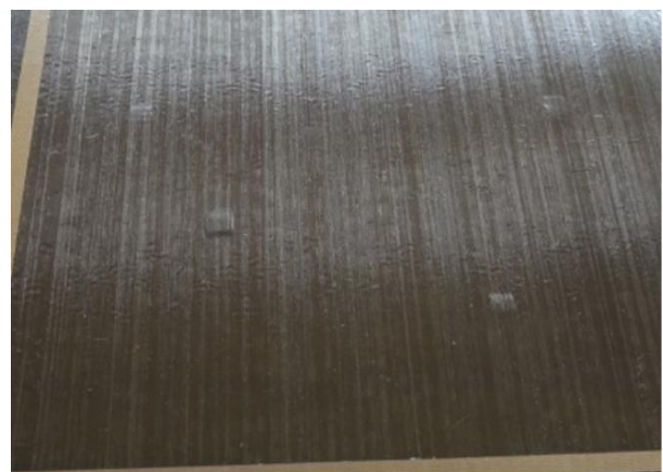
Fig. 4 Thickness variation on the top surface due to inclusions
