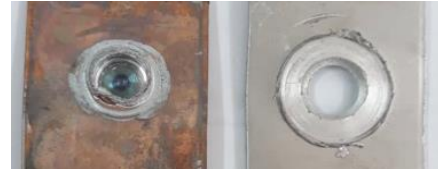
Fig. 8 Shear failure of the weld at the joint interface of two sheets.
