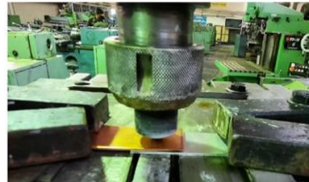
Fig. 4 Fixtures and clamps for welding specimens.
