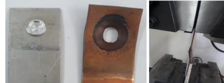
Fig. 7 Nugget fracture after high energy absorption.
