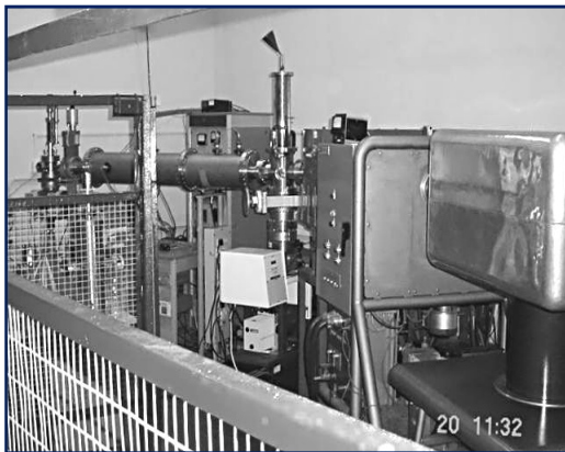
Fig. 2 Setup of 150 keV ion implanter
