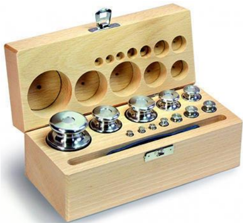
Fig. 9(u) This is the set of standard weights that we used for the calibration.
