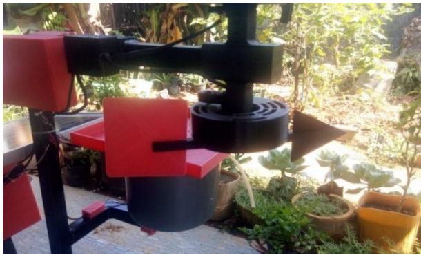
Fig. 2 (c) This is the 3D printed and assembled wind direction sensor
