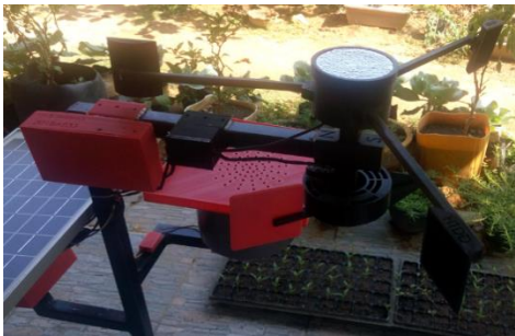
Fig. 1 (c) The actual sensor that was 3D printed and assembled is shown here.
