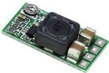
Fig. 7 (c) The buck converter, which can adjust its voltage, or by soldering the appropriate jumper, we can generate a very stable and consistent voltage.
