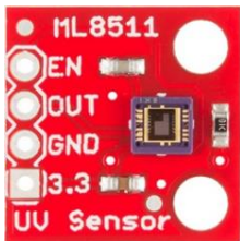
Fig. 6 (a) ML 8511 is a UV sensor; it needs a reference voltage to work, and the given voltage output is converted to UV index by using a microcontroller.
