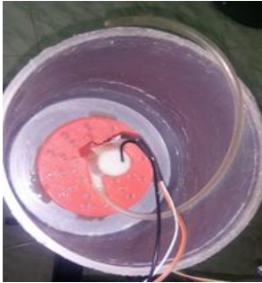
Fig. 3 (a) This shows the inside mechanism of the sensor. There is a water level sensor, a submerging pump, and a water particle filter.
