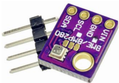
Fig. 5 (a) BME 280 is an I2C communication base multivariable sensor.
