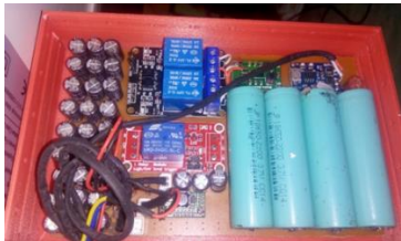
Fig. 8 (a) Assembled power circuit: There are three relays; one is used for power output battery or solar, and the other two are used to charge and discharge the batteries. There are two buck converters, one is used for solar panel voltage to 5 V, and the other is used to convert battery voltage to 5 V. The capacitor banks help to supply power when the circuit voltage changes.
