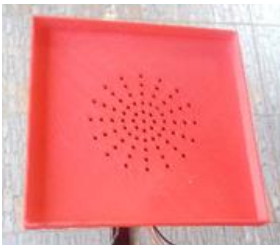
Fig. 3 (b) This is the water collecting bin which used to collect rainwater in the area of 200 mm × 200 mm. There is a particular filter that can remove particles such as leaf insects, etc.
