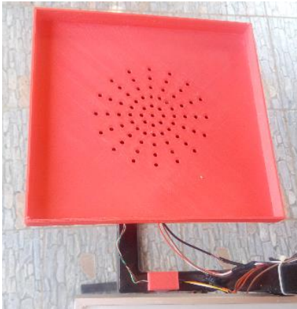
Fig. 9(v) This is the water collection bin in the rain gauge. This is the area we have used to put weights for calibration.
