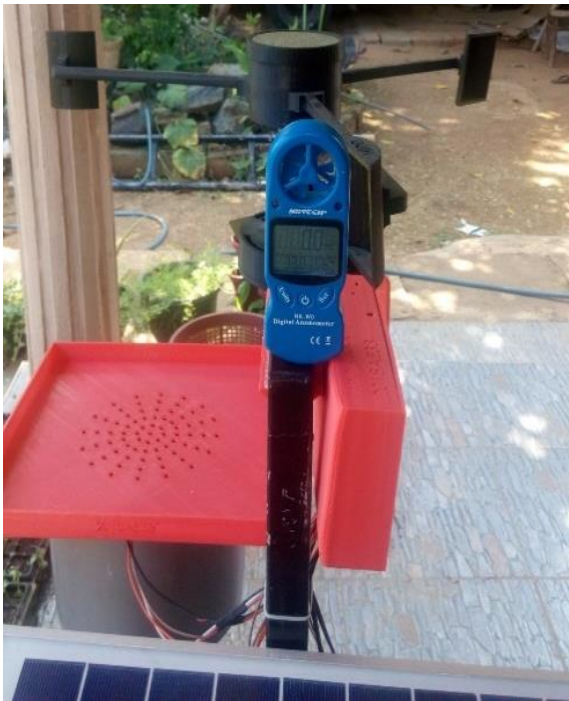
Fig. 9(s) shows the Calibration for the wind speed setup. We used a glue tap to hold the anemometer and a fan to create different wind speeds.
