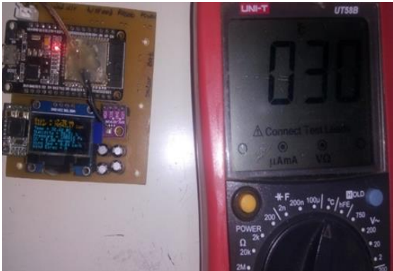
Fig. 9 (d) This is the temperature calibration setup for the BME 280 sensor. A K-type multimeter temperature probe is attached to the sensor using glue. Collect sensor readings on OLED display, and temperature readings of K-type sensor are collected using a multimeter.
