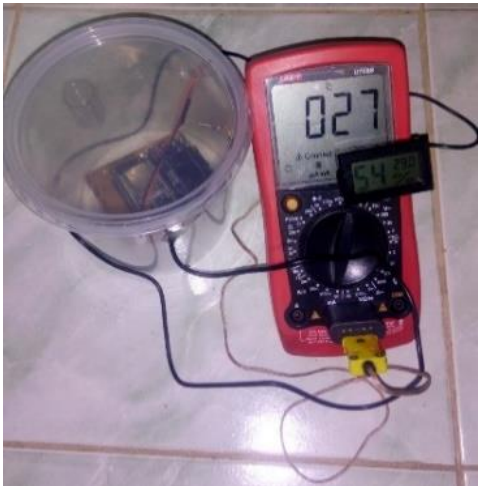
Fig. 9 (i) This is the overall setup of the humidity calibration. To measure humidity, we used BME 280 and an industrial available instrument, and for temperature, we used the same items and a multimeter with a K-type sensor.
