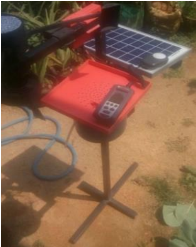
Fig. 4 (a) This is the calibration setup of solar light intensity. Sensor data and LUX meter readings are recorded.
