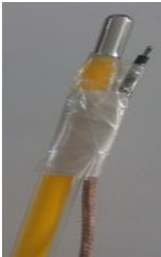
Fig. 9 (e) connecting a K-type thermal sensor to a mercury thermometer for calibration.
