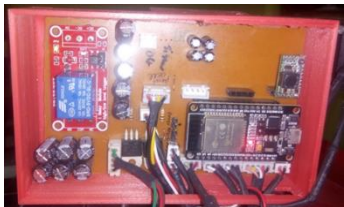
Fig. 8 (b) This is the main control circuit. There is an ESP 32 as the main controller, a buck converter as a voltage converter that uses 5 V to 3.3 V. The Relay module is used to turn on and off the water pump. TIP 120 transistors are used
