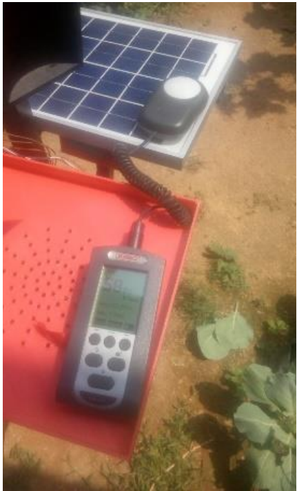
Fig. 9(p) This is the Calibration of solar light intensity. Put the solar panel and light meter sensor simultaneously and get the same reading.
