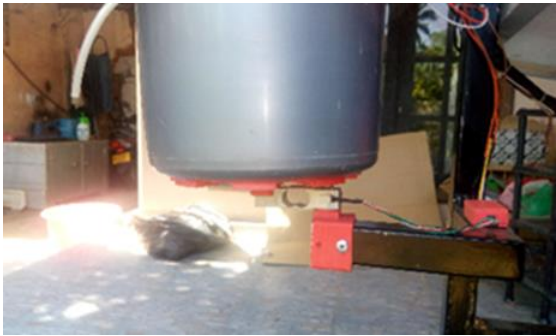
Fig. 3 (d) The water collecting bin is on the load cell, and it is permanently attached to the instrument body by using a nut and bolt.
