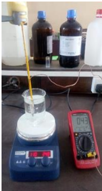
Fig. 9 (f) This is the overall multi-meter calibration setup. By increasing the water temperature, multi-meter and thermo meter readings are recorded.
