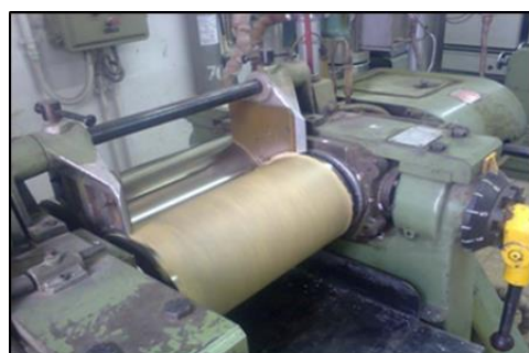
Fig. 2. Elaboration of PVC/MMT Nanocomposites Using a Twin-roll Mixer
