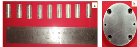
Fig. 2 a) Wear test specimen b) Counterpart disc
