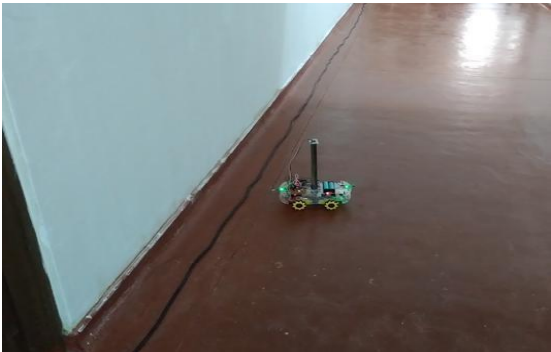
Fig. 9 The robotics car navigated and started to collect magnetic field sensor readings.
