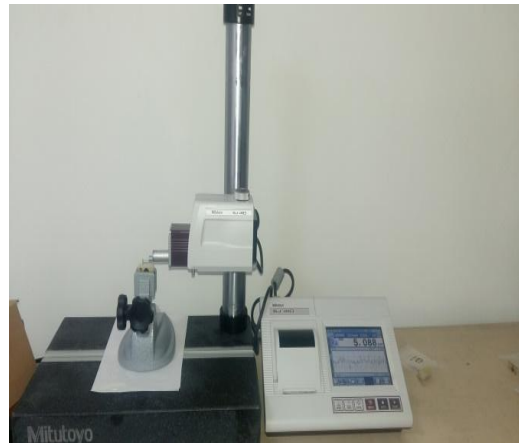
Fig. 3 Surface roughness tester (Model -Mitutoyo SJ-210)
