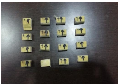
Fig. 2 Machined work piece samples of Kevlar epoxy composite
