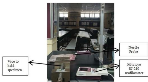
Fig. 1. Experimental Setup for Surface Roughness Measurement
