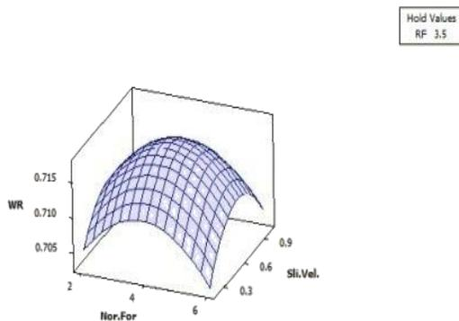
**Fig.2 Influence of Normal Force and RF on WR and Sliding Velocity on WR**
