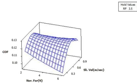
**Fig.4 Influence on Normal Force RF of COF and Sliding Velocity on COF**
