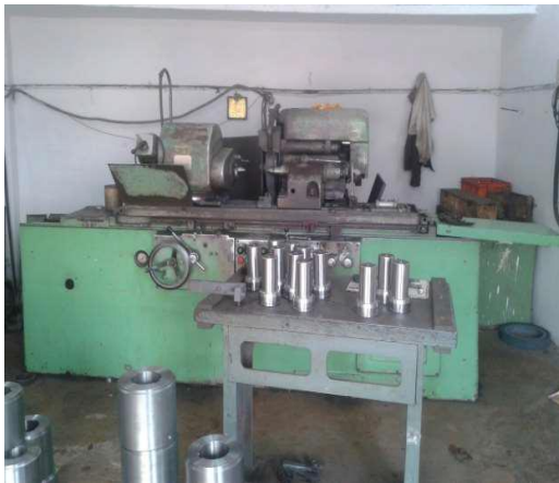
Fig. 1 Cylindrical Grinding Machine HMT G17 800
