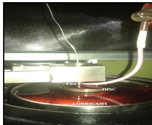
Fig. 2 Experimental setup with WINDUCOM software
