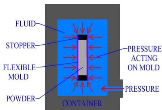
Fig. 3 Principle of Iso static pressing
