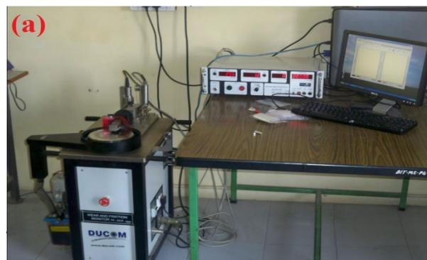
**Fig. 6 Pin-on-Disc wear testing apparatus**
