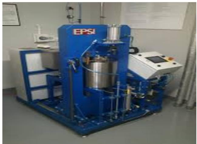
Fig. 2 Iso static pressing Machine
