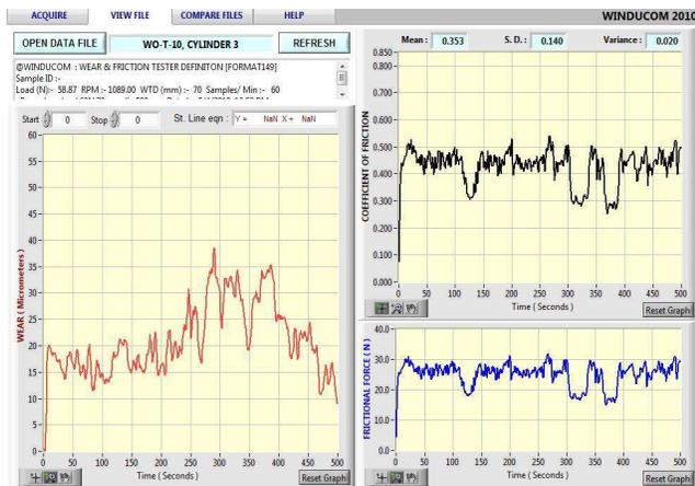
Fig. 9 Wear rate for Cylinder 3-1 (a. wear v/s Time b.cof v/s Time c. frictional force v/s Time )
