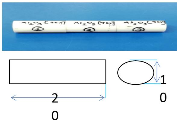
**Fig. 5 Wear Test Specimen**
