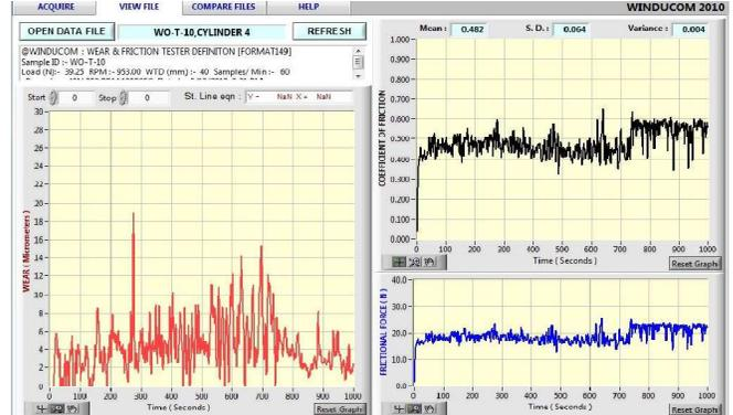
Fig.10 Wear rate for Cylinder 3-2 (a. wear v/s Time b.cof v/s Time c. frictional force v/s Time)
