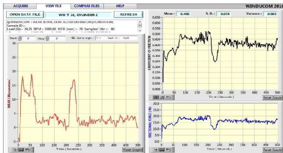
Fig. 8 Wear rate for Cylinder 2-1 (a.wear v/s Time b.cof v/s Time c. frictional force v/s Time)
