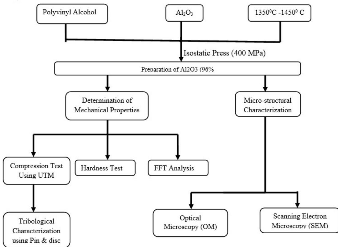
Fig .1Pure Al<sub>2</sub>O<sub>3</sub>material testing flow chart
