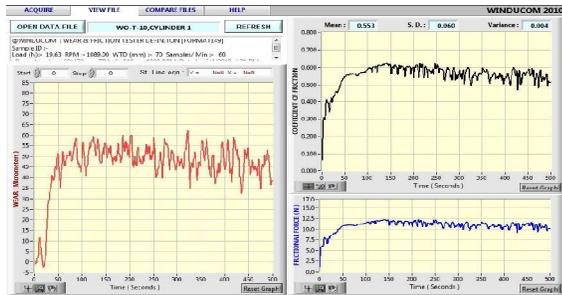
Fig. 7 Wear rate for Cylinder 1-1 (a wear v/s Time b.cof v/s Time c. frictional force v/s Time )
